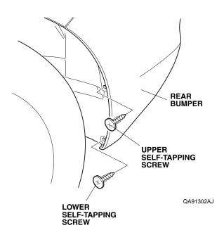
Insert the top edge of the left bracket behind the inner fender, and reinstall the upper self-tapping screw.
