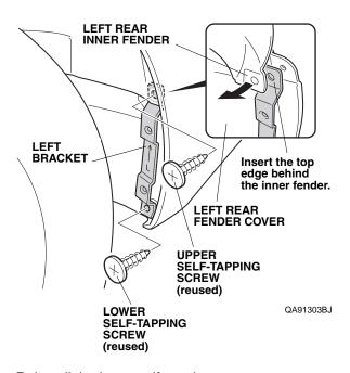
7. Reinstall the lower self-tapping screw.
